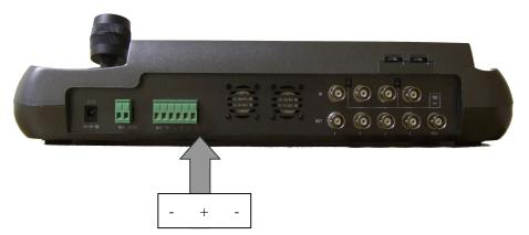
Connect the RS485 data cable to the connections on the rear of the keyboard (see diagram above). Note that the orange connection is the RS485 + A Line connection and the yellow is the RS485 - B Line connection. Note that there are two sets of RS485 connections.
