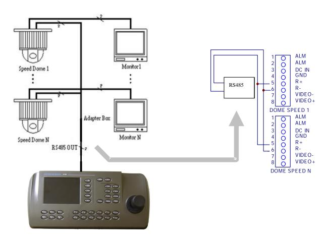
Note: As the protocol and baud rate of the dome camera are set by menu in this keypad, multiple domes must use the same protocol and baud rate.
